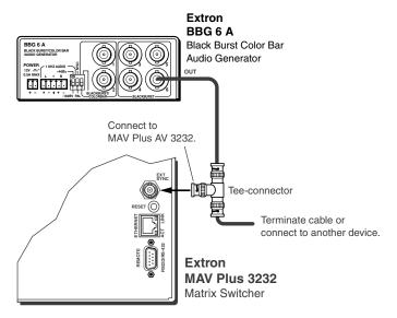
Figure 2-22 — Simple external sync connection example
